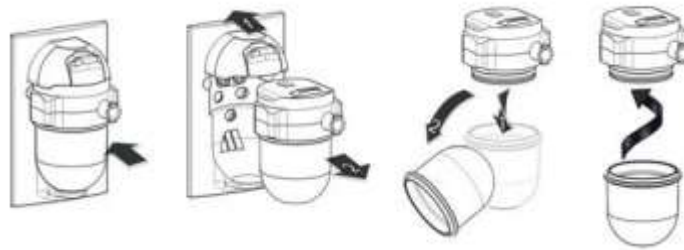
Figure 1.6 – Emptying of a water trap
